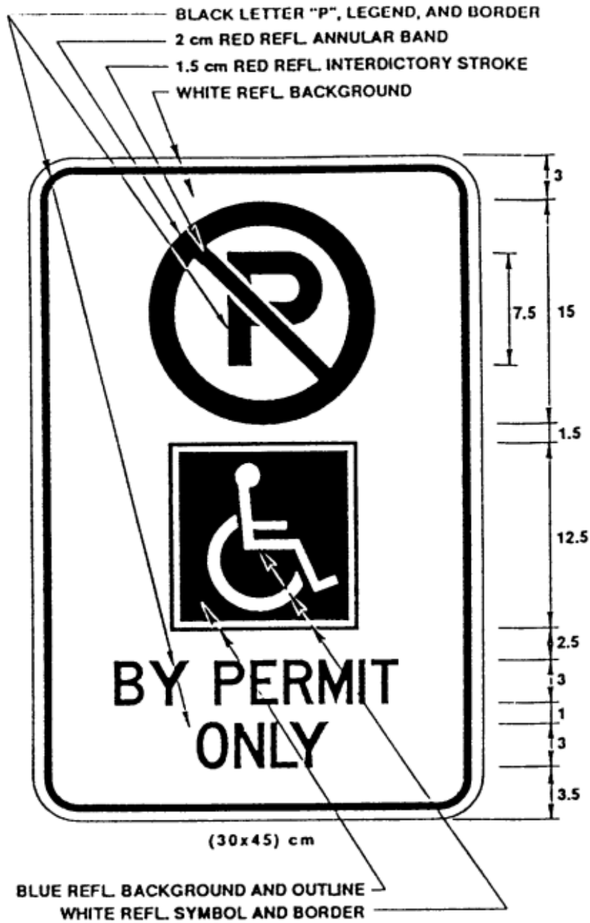
Figure 1: Standard post signage for designated accessible parking spots (source: O. Reg. 308/10, s.11)
