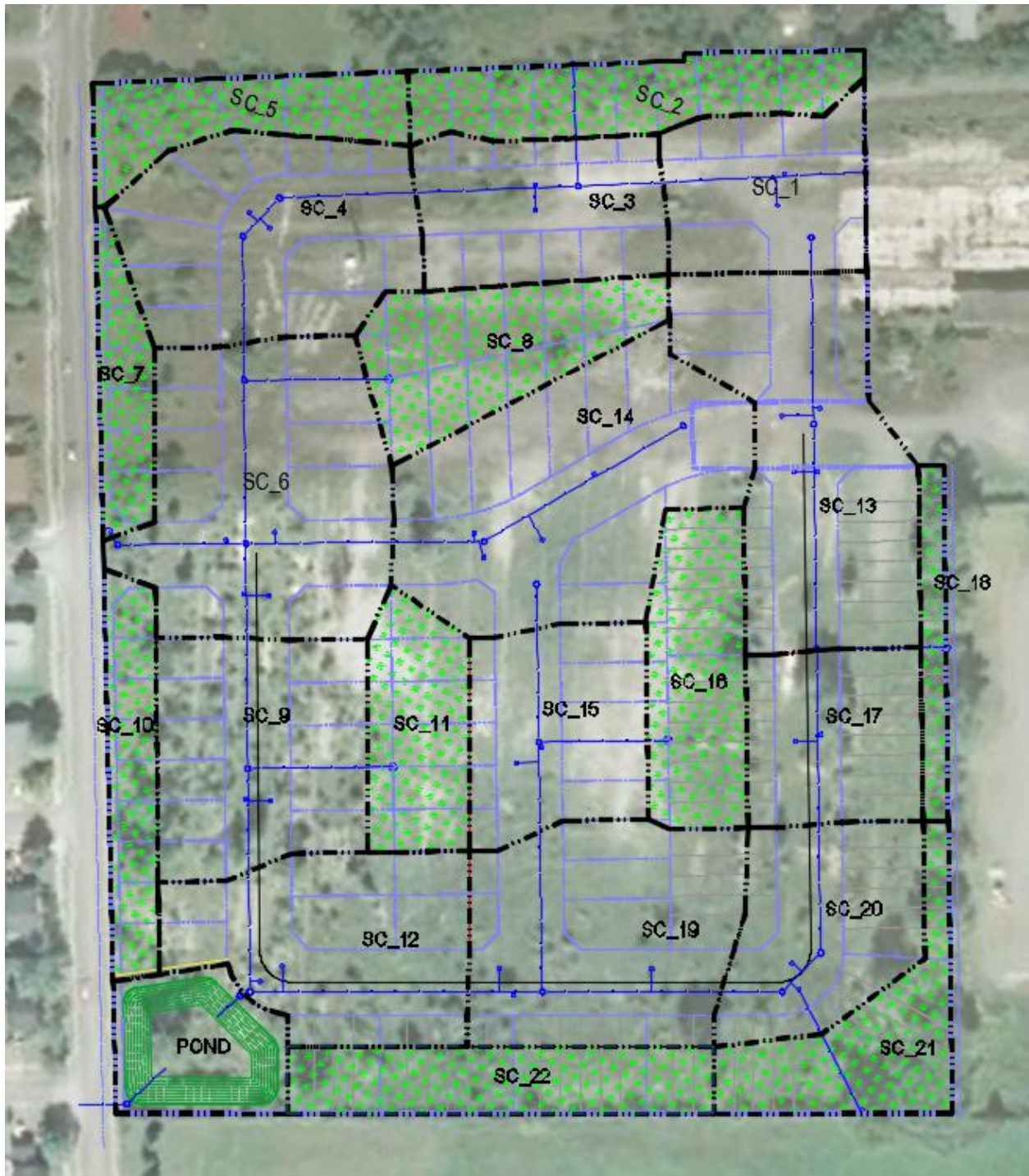
Figure 4-1: Post-Development Sub-Catchment Boundary
