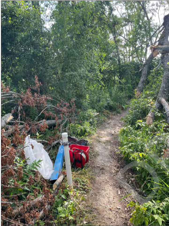
Photo 1 – Damaged well casing looking northeast located on the southwest side of the property – MW157. July 11, 2022
